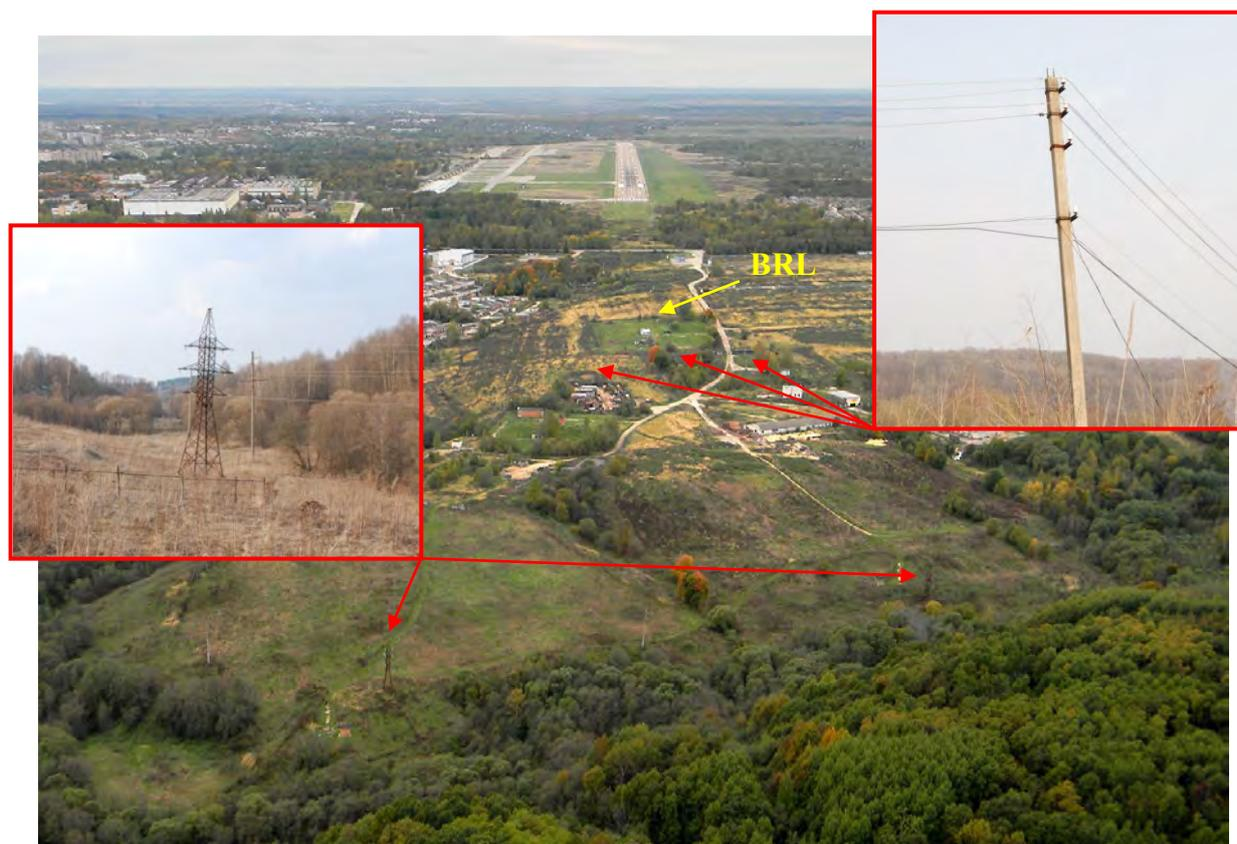
Photo 17. Location of power lines and low-voltage lines relative to Inner NDB
