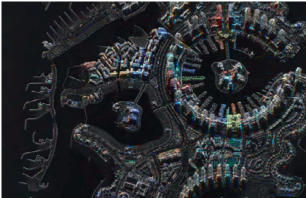
Accurate, near real-time Earth monitoring with SAR data. Dwell Mode CSI (Colorized Subaperture Image) emphasizing man-made objects using various colors
